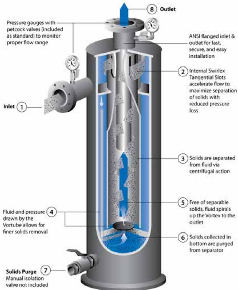
LAKOS Separators are designed specifically to remove solids from liquids. Each model is calculated for use within a prescribed flow range for maximum performance and solids removal. Flow rates above and below the recommended range may affect such performance.
